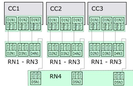
Other variants of how a single 3-node **FireTrac®** card can be used are depicted below. The left shows a CC devices simulating the triple bus interface (3 CC) whereas the right pictures demonstrates a possible single-branch usages model (CC + 2 RNs).
