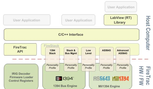
The *Personality Profiles* allow the solution to be adapted for use in embedded systems which typically have limited resources, and/or with powerful host processors that can utilize even the fully featured profile.
