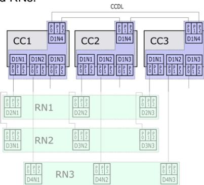
However, the above is only an implementation variant. A 4-node **FireTrac®** can also be used to simulate single branch bus behavior (left and middle) or mixed CC/RN situation in double redundancy (right).
